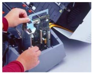
6. Attach and tighten the fourth thumbscrew on top of the circuit board mounting bracket.
